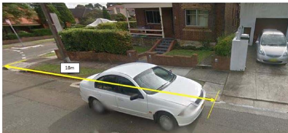
Photo 5. Robert Street at Victoria Street, Ashfield – Illegal parked vehicles less than 10 meters from this intersection. Extend 'No Stopping' to 18 meters to clear traffic passage between corner and central splitter island to roundabout.
