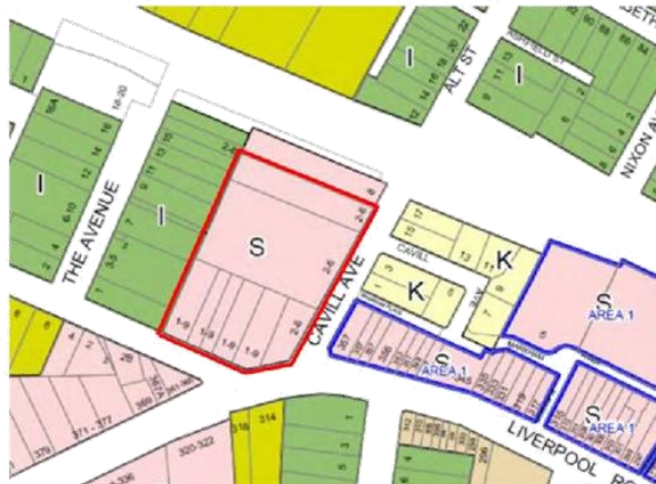
Figure 2 - Extract Ashfield LEP 2013 – Maximum Building Height Map. Code S signifies 23 metres, Code I signifies 8.5 metres, Code K signifies 10 metres. Blue boundary indicates where a 7 metre height bonus applies.
