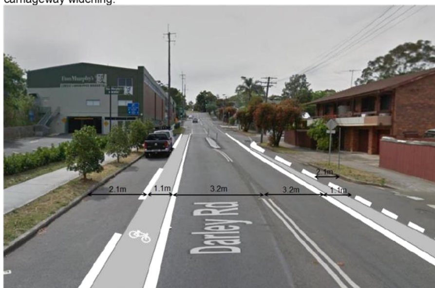
Figure 5: typical example of separated unidirectional cycleway and work required in Darley Rd.
