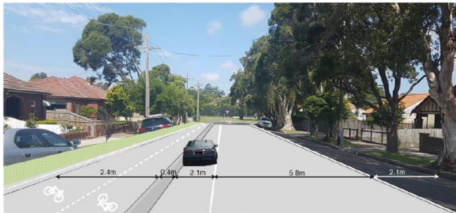
Figure 18: typical example of separated bi-directional cycleway and retained parking on both sides of the road.
