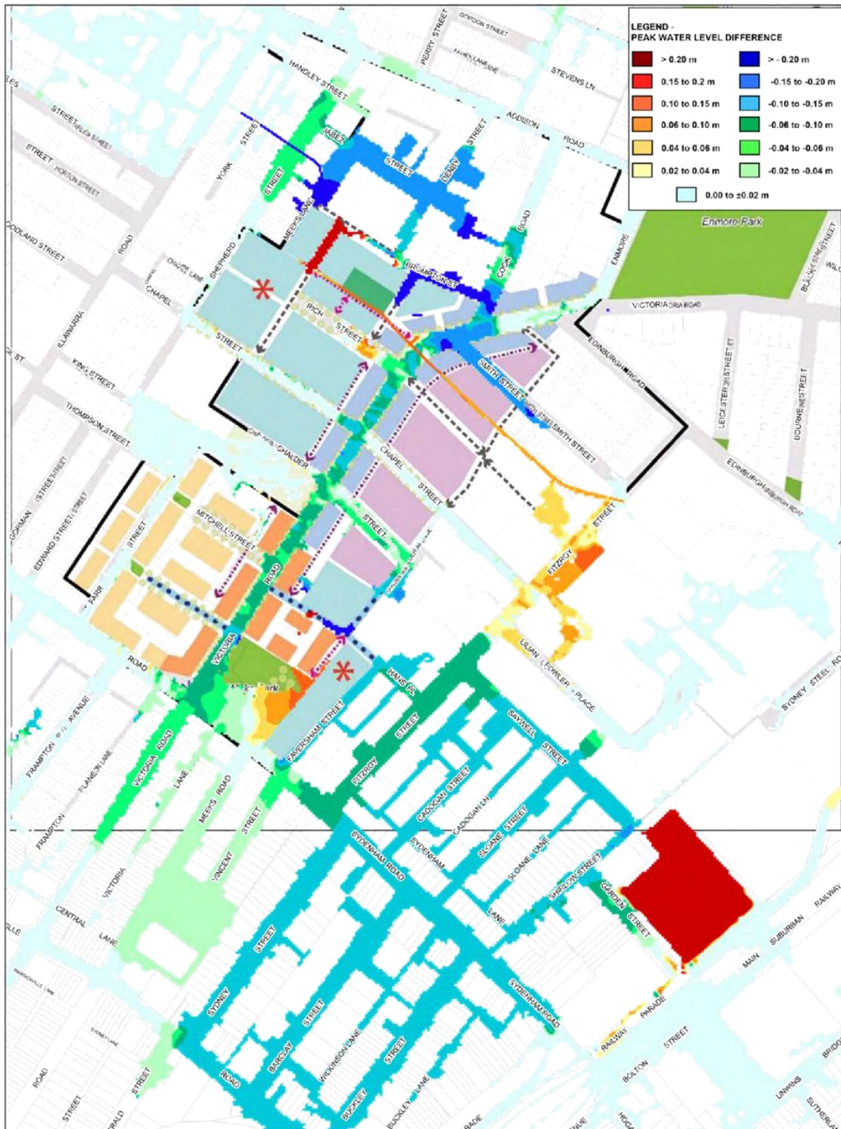
VICTORIA ROAD PRECINCT Design Scenario- Option 4 Water Level Difference (Option 4 Less Existing)
