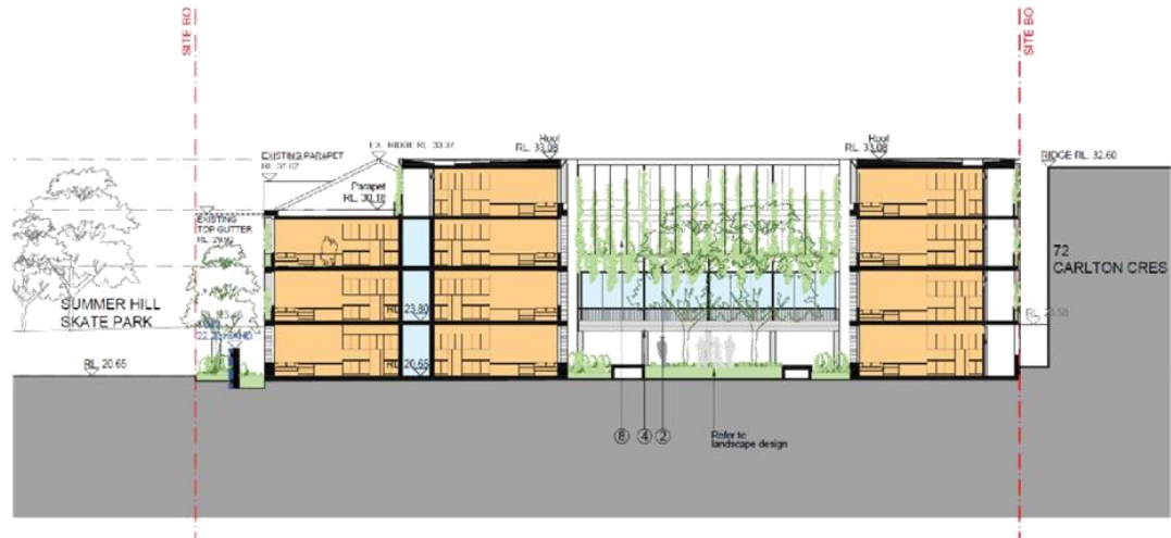
Figure 4: Revised east west section plan showing the flood wall to the western boundary
