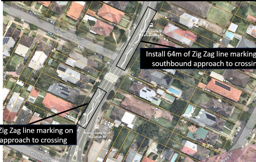
Zig Zag line markings to be installed as per above
