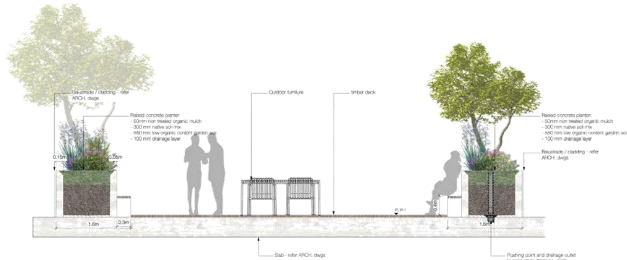
E Communal space roof (L7) Section - Scale 1:25
