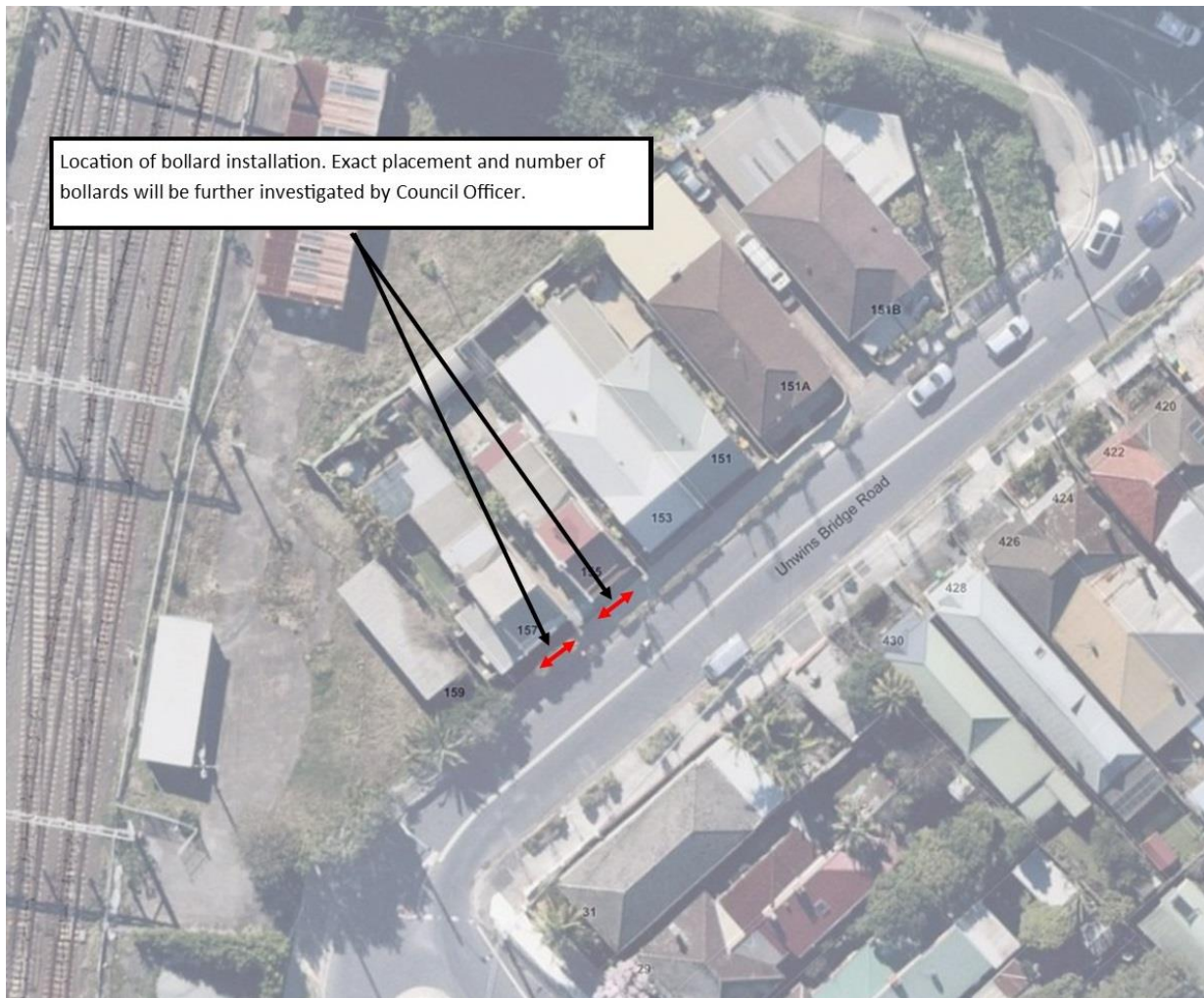
Diagram 2: Concept Plan for installation of bollards along frontage of Property No. 155 & 157 Unwins Bridge Road, Tempe.
