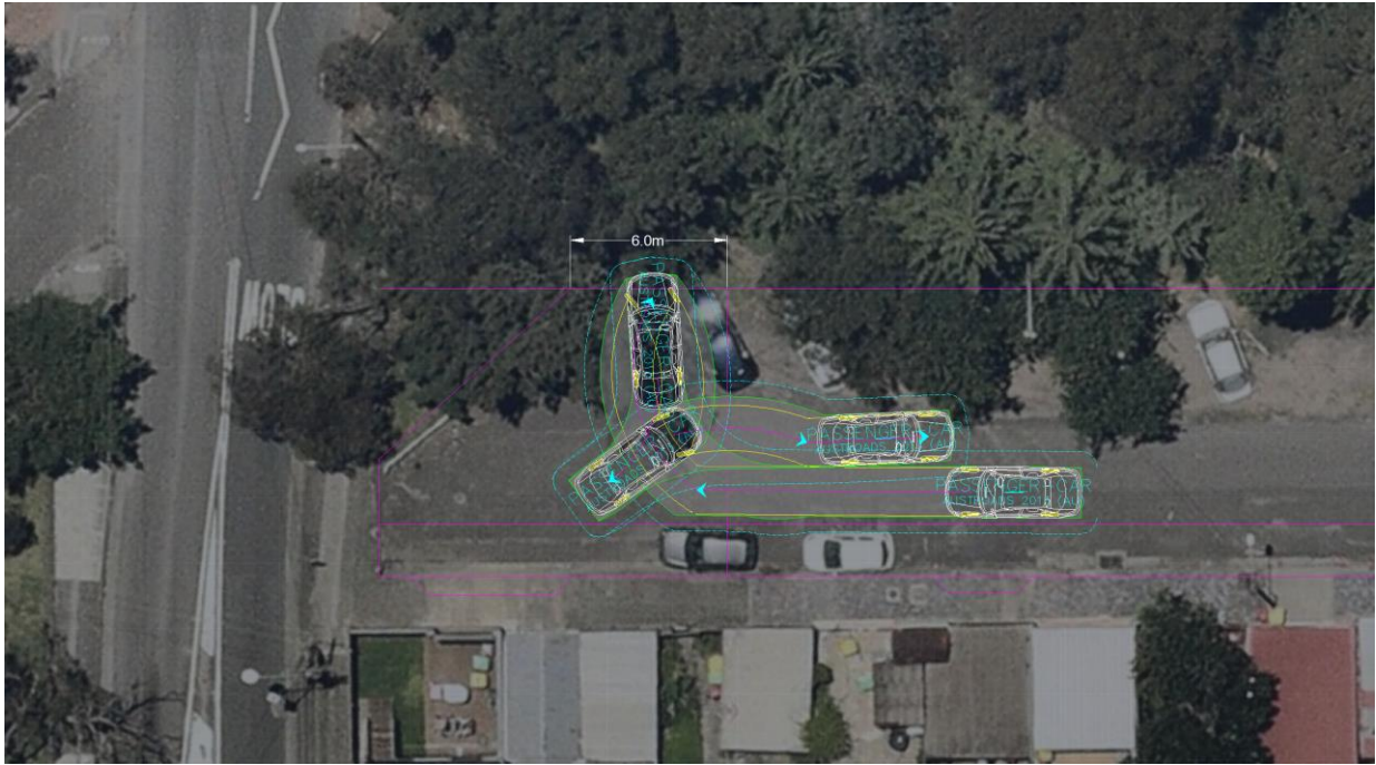
Figure 3 - Swept path 1 - Turn around movement at dead-end
