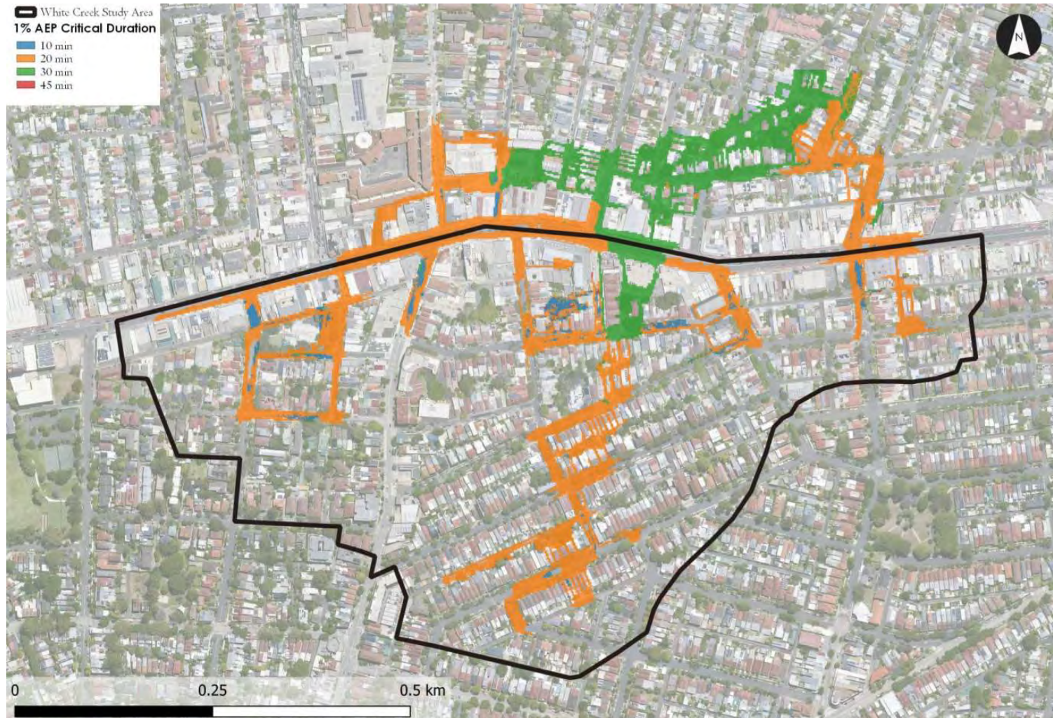
Figure 3-7 1% AEP Critical Duration Storms for Updated Model for Whites Creek Study Area Based on AR&R 2019 Design Rainfall Updates
