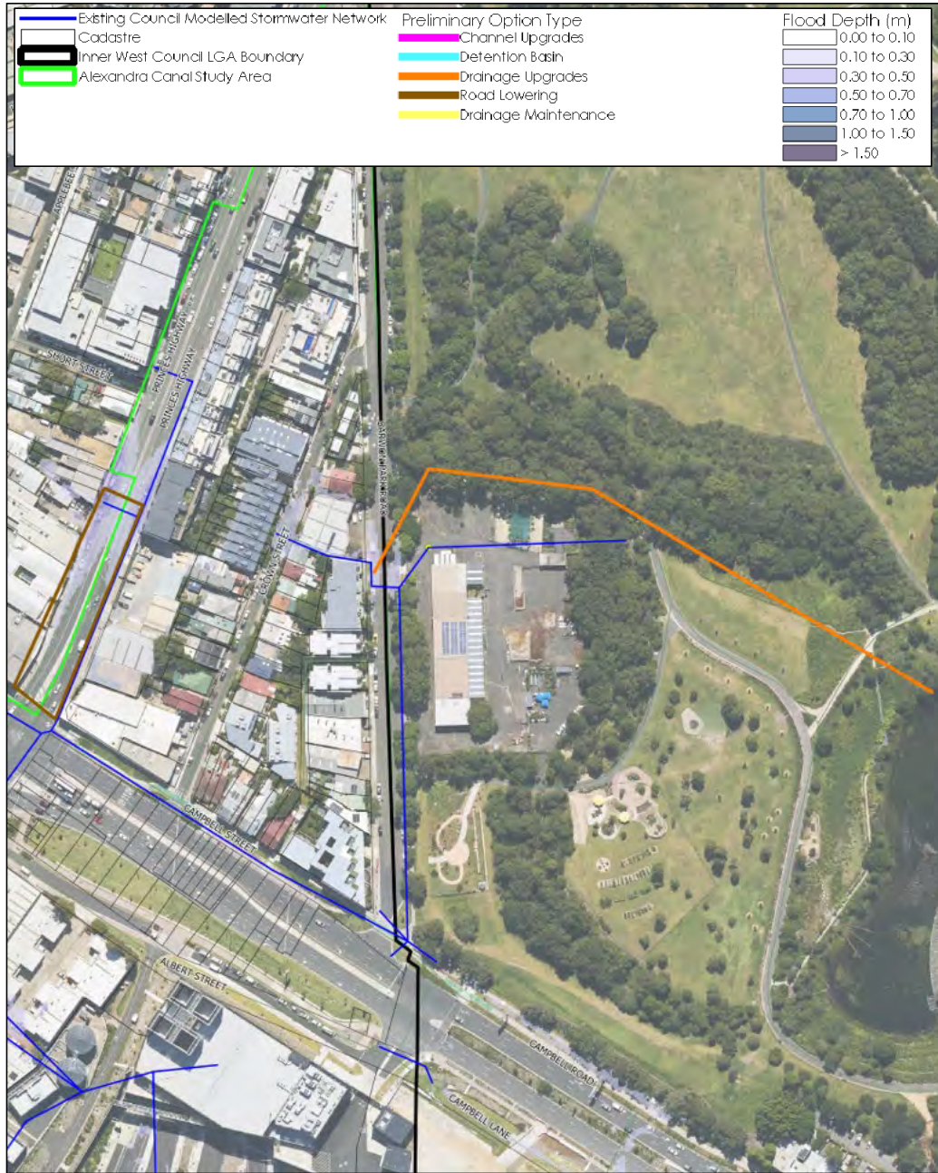
Figure 8-3 Alexandra Canal Hotspot 3 Preliminary Mitigation Options with 1% AEP Existing Peak Depth Results
