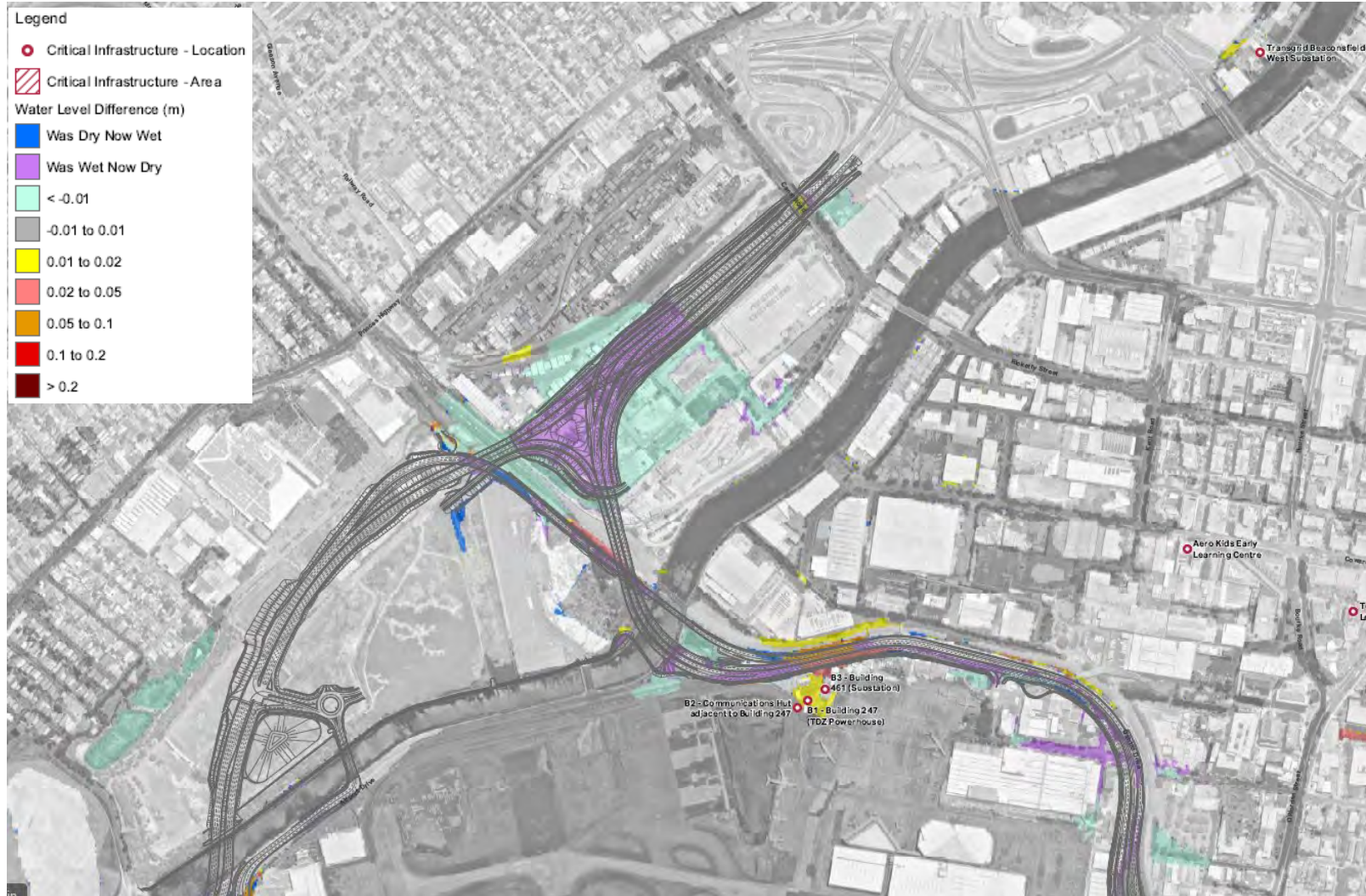
Figure 2-11 1% AEP Water Level Event Impacts of the Sydney Gateway Project within the Study Area (Sydney Gateway JV, 2021)
