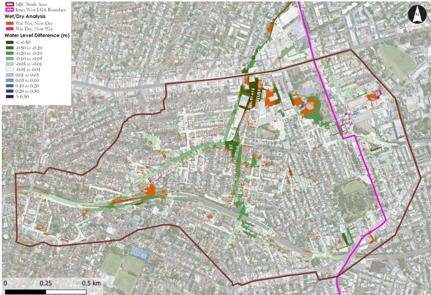
Figure 3-6 5% AEP Peak Water Level Differences – Johnstons Creek - Updated AR&R 2019 Model Less Flood Study AR&R 1987
