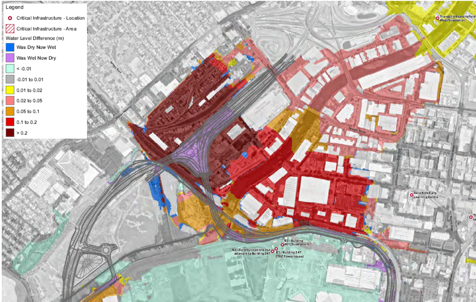
Figure 2-12 PMF Water Level Impacts of the Sydney Gateway Project within the Study Area (Sydney Gateway JV, 2021)
