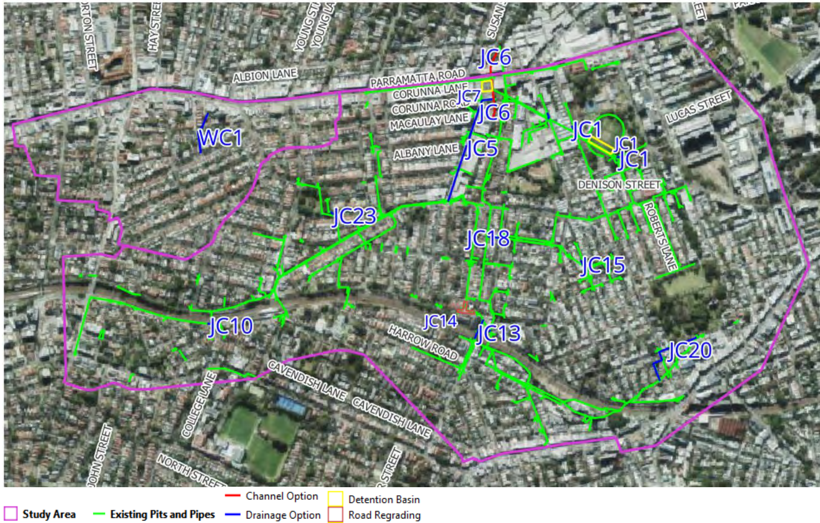
Figure 9-1 Location of 14 Detailed Flood Modification Options for Whites Creek and Johnstons Creek
