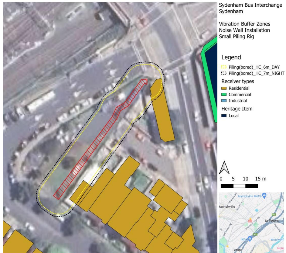
Figure 6-25 Vibration buffer zones – noise wall installation - small piling rig
