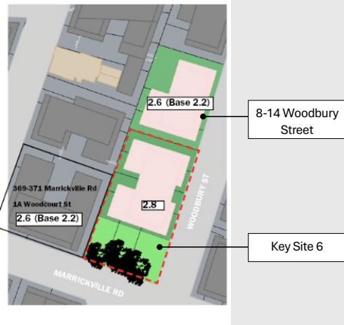
Key Site 6 and assumed amalgamated 8-14 Woodbury Street site – Amended indicative Plan and proposed built form controls indicating the FSRs
