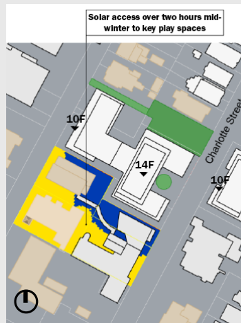
Solar access analysis of the adjoining St Vincent Catholic School from one of the indicative building envelopes tested at 40 Charlotte Street.
