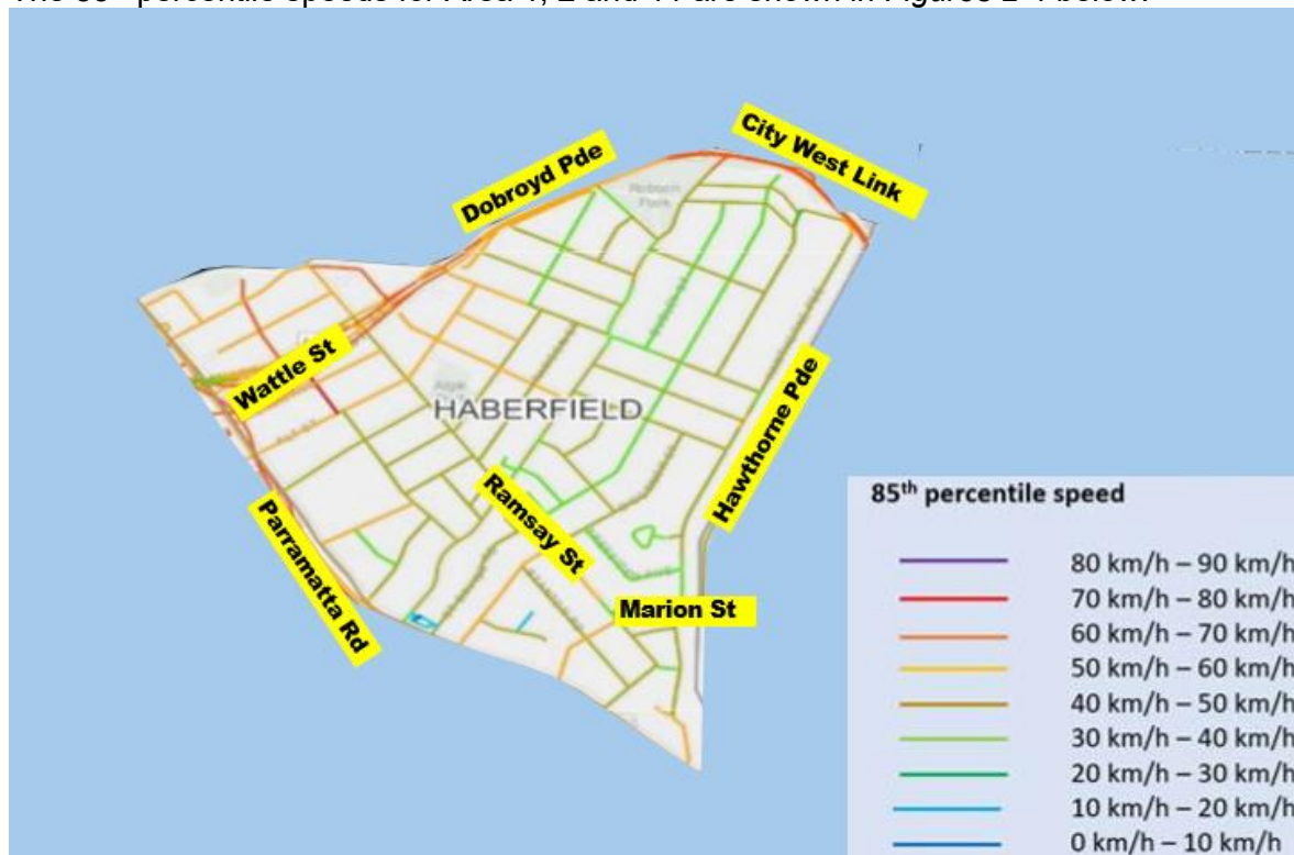
Figure 2: 85 th percentile speed profile for Haberfield (area 1)
